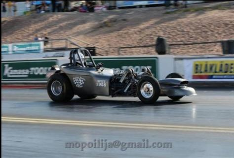
From zero to 270 km/h in 7.9 seconds and just in 402 meters of travel. That is our target and to do that, we will need about 800 horsepower!
